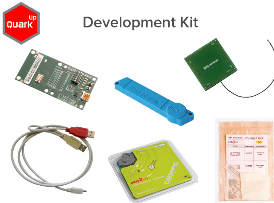
Fig. 1.4: R1270CXDK: Accessories kit with adapter, antennas, cable and demo tags
