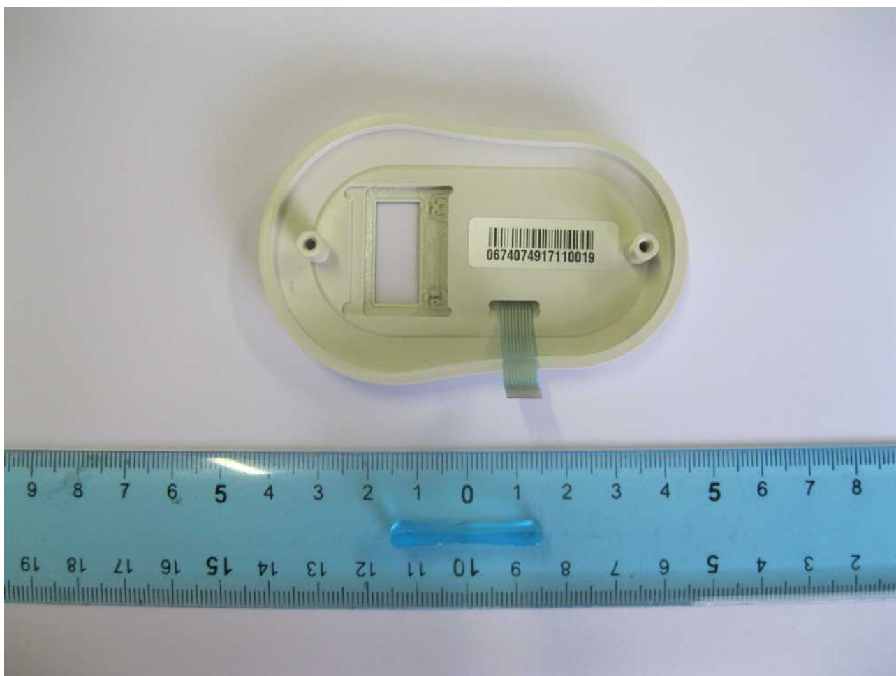
Fig. 8: Enclosure and keypad Top Side (internal view)
