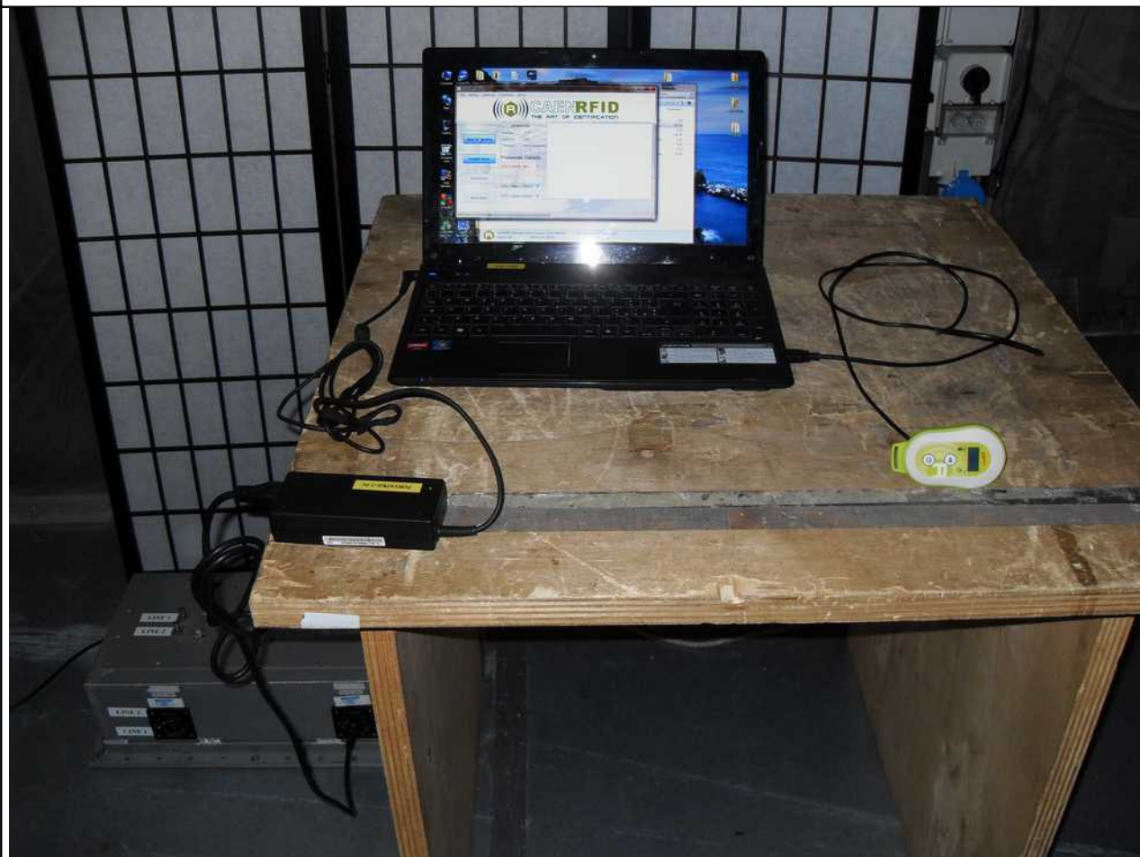
Fig. 6.1 Conducted Emissions Test Set-up
