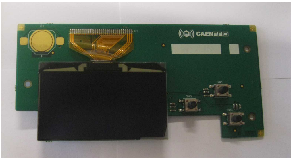
Figure 6: Display Board – Top side
