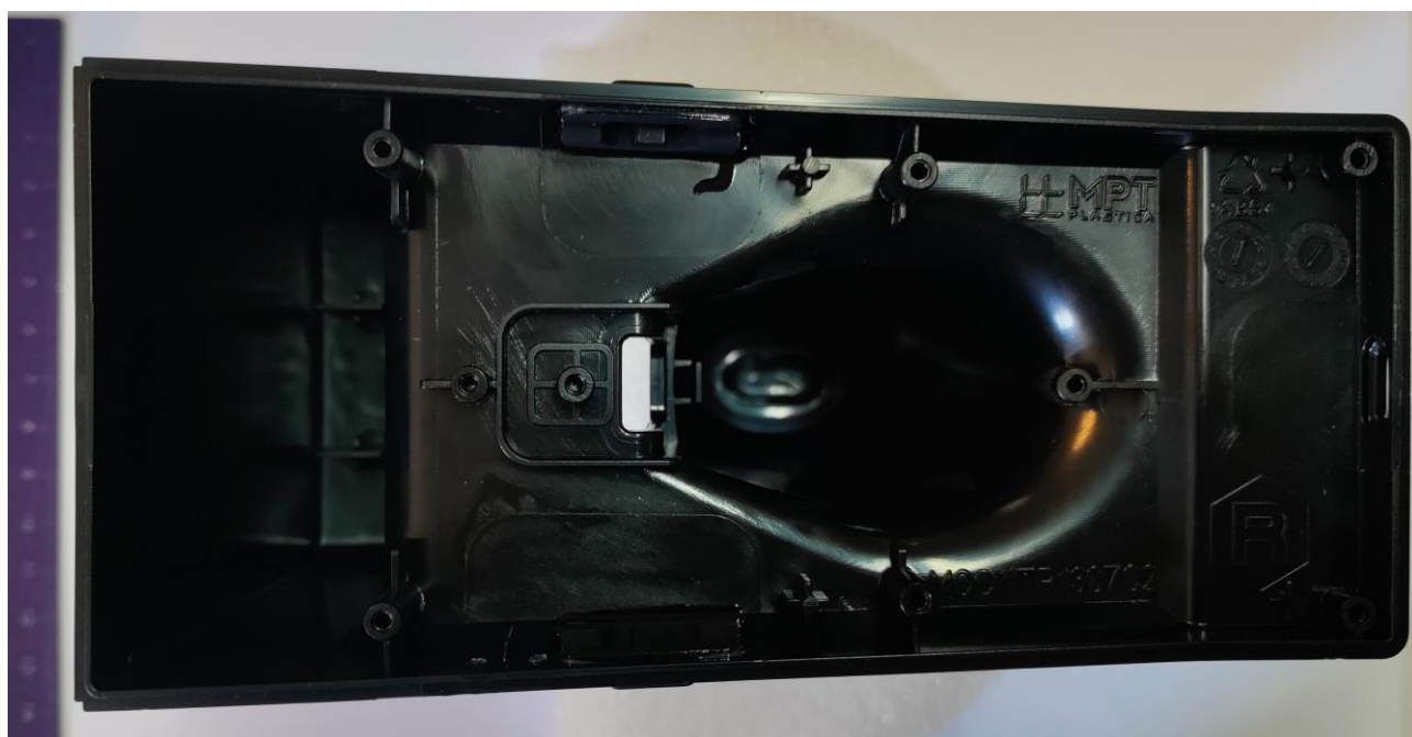
Figure 14: bottom enclosure – internal view
