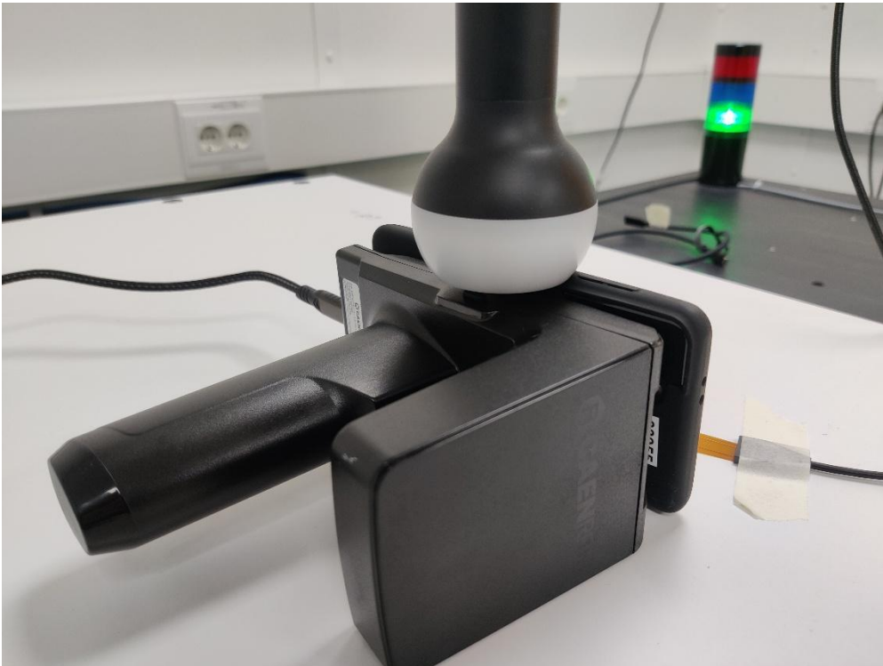
Figure 10. Left side of the DUT with a separation distance of 0mm
