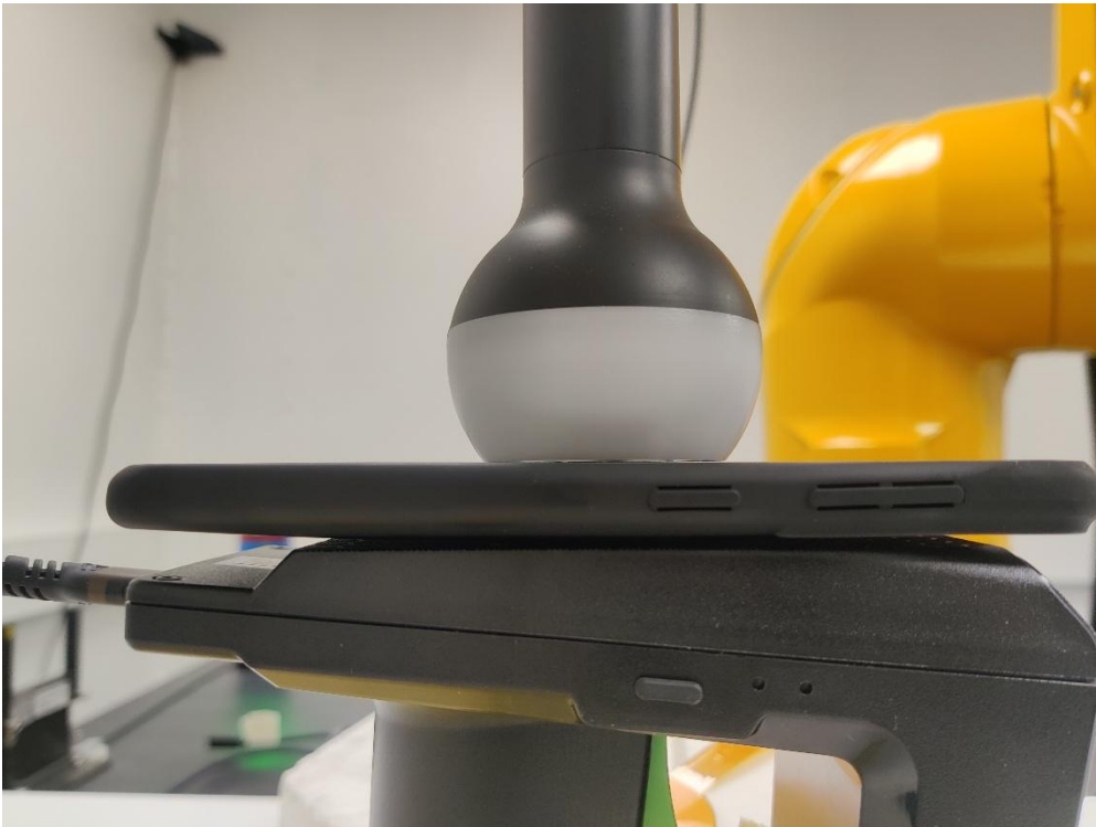
Figure 8. Top side of the DUT with a separation distance of 0mm
