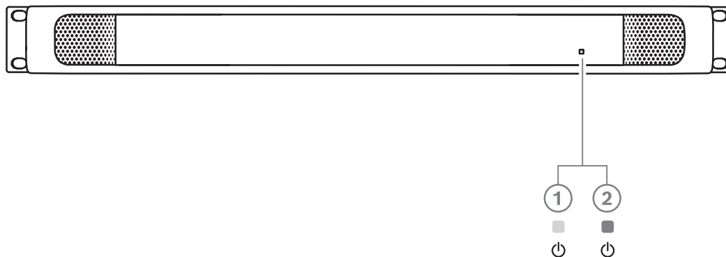
Figure 6.6: OMN-DANTEGTW front panel description
