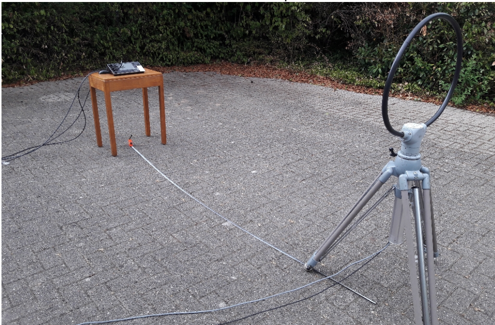
Radiated emissions test setup below 30 MHz
