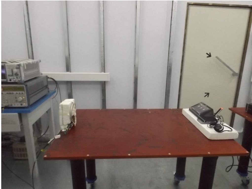
Photograph 4: Set-up for Conducted Emission testing
