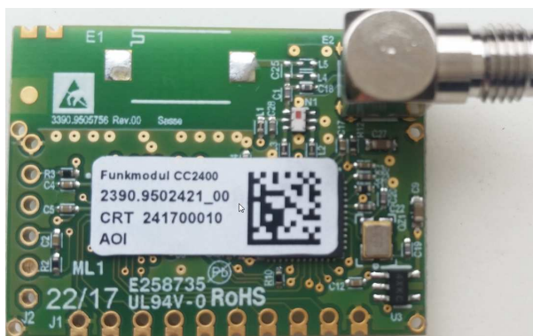
Fig. 2: Transceiver module TM2.4-2 (with external antenna)
