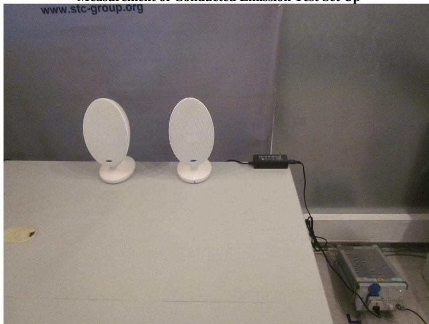
Measurement of Conducted Emission Test Set Up
