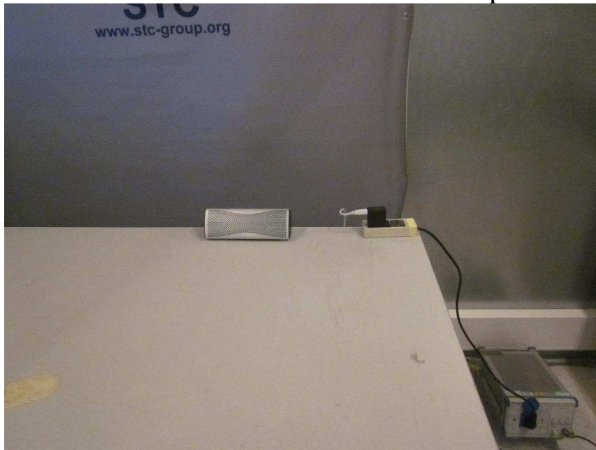
Measurement of Conducted Emission Test Set Up
