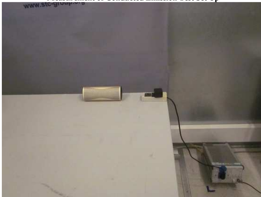
Measurement of Conducted Emission Test Set Up
