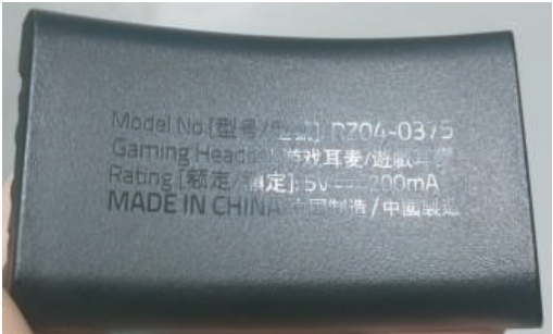
Reference sample of the mold etching high gloss effect
