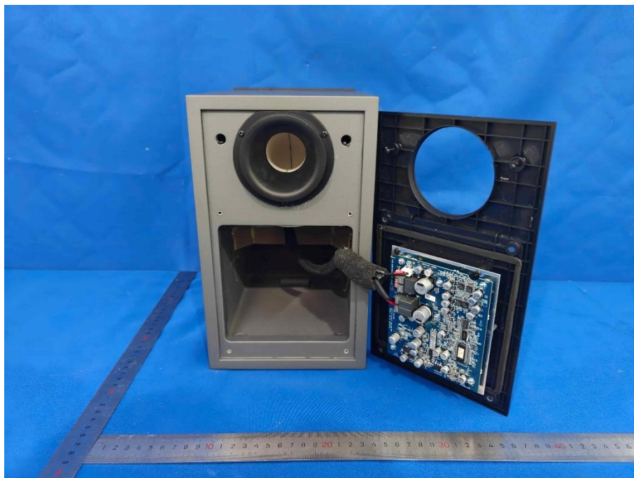
Figure 25: Secondary Speaker Internal View
