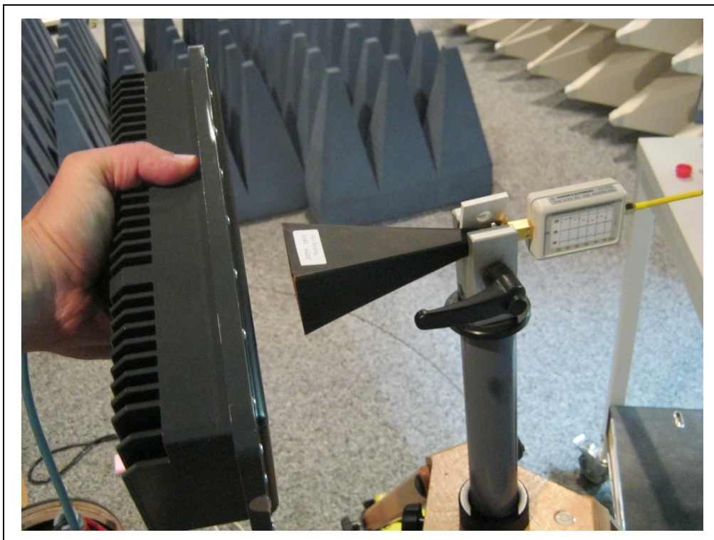
Photograph A1-12: Radiated emissions 50 – 75 GHz at close distance
