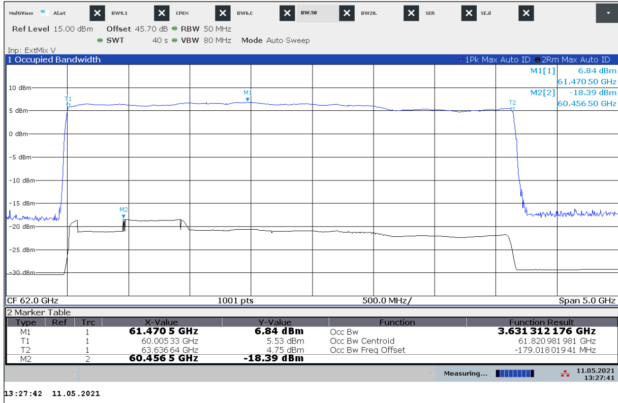
Plot 42: Frequency Stability, Single Target Mode (STM), 20 °C / V min-max
