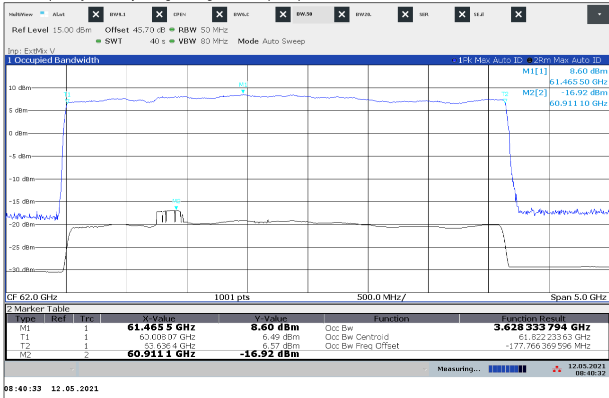
Plot 43: Frequency Stability, Single Target Mode (STM), 30 °C / V min-max
