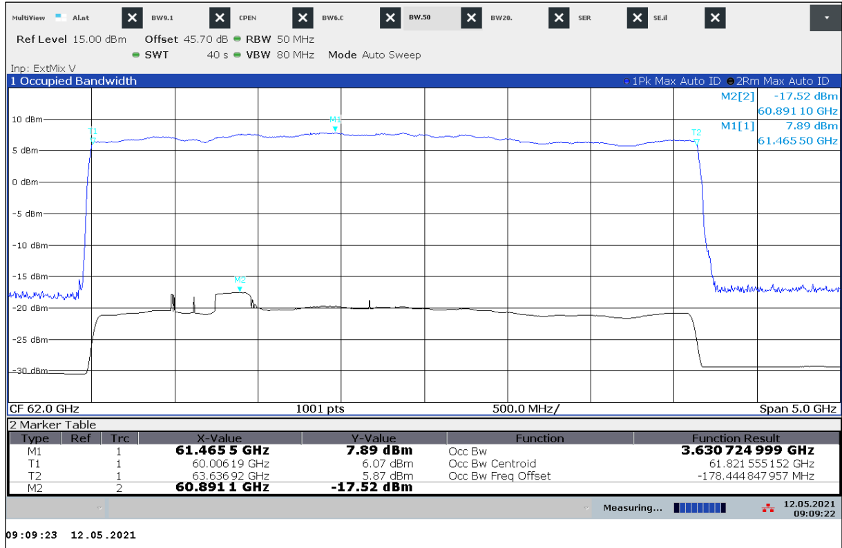
Plot 44: Frequency Stability, Single Target Mode (STM), 40 °C / V min-max
