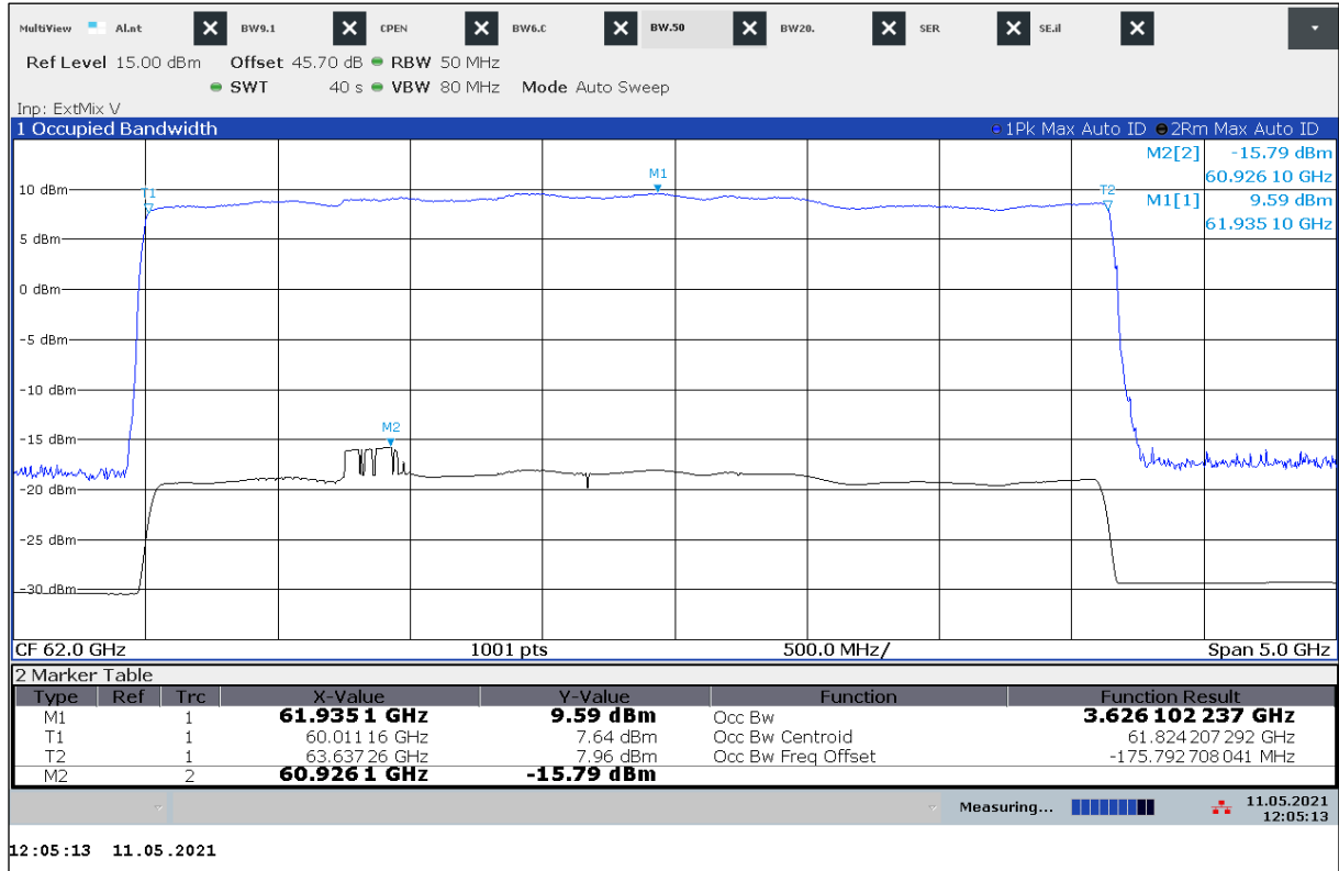
Plot 38: Frequency Stability, Single Target Mode (STM), -20 °C / V min-max
