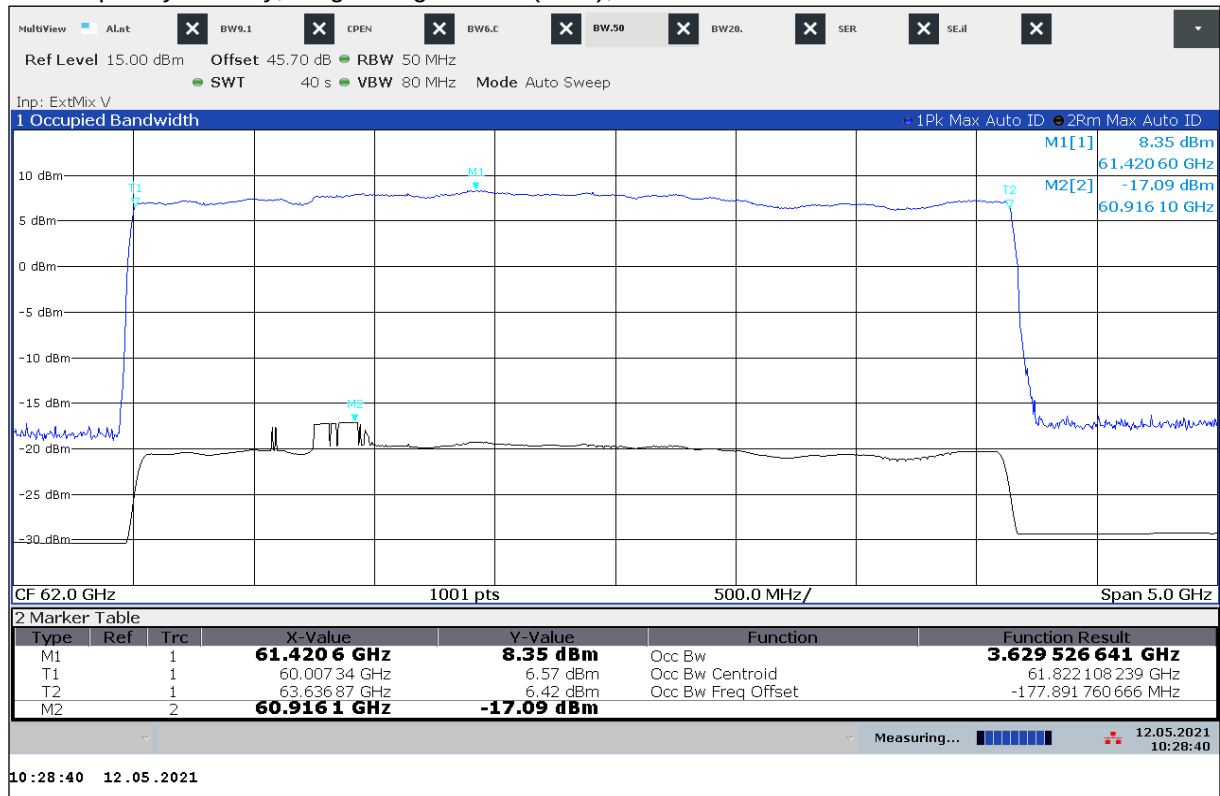
Plot 46: Frequency Stability, Single Target Mode (STM), 85 °C / V min-max
