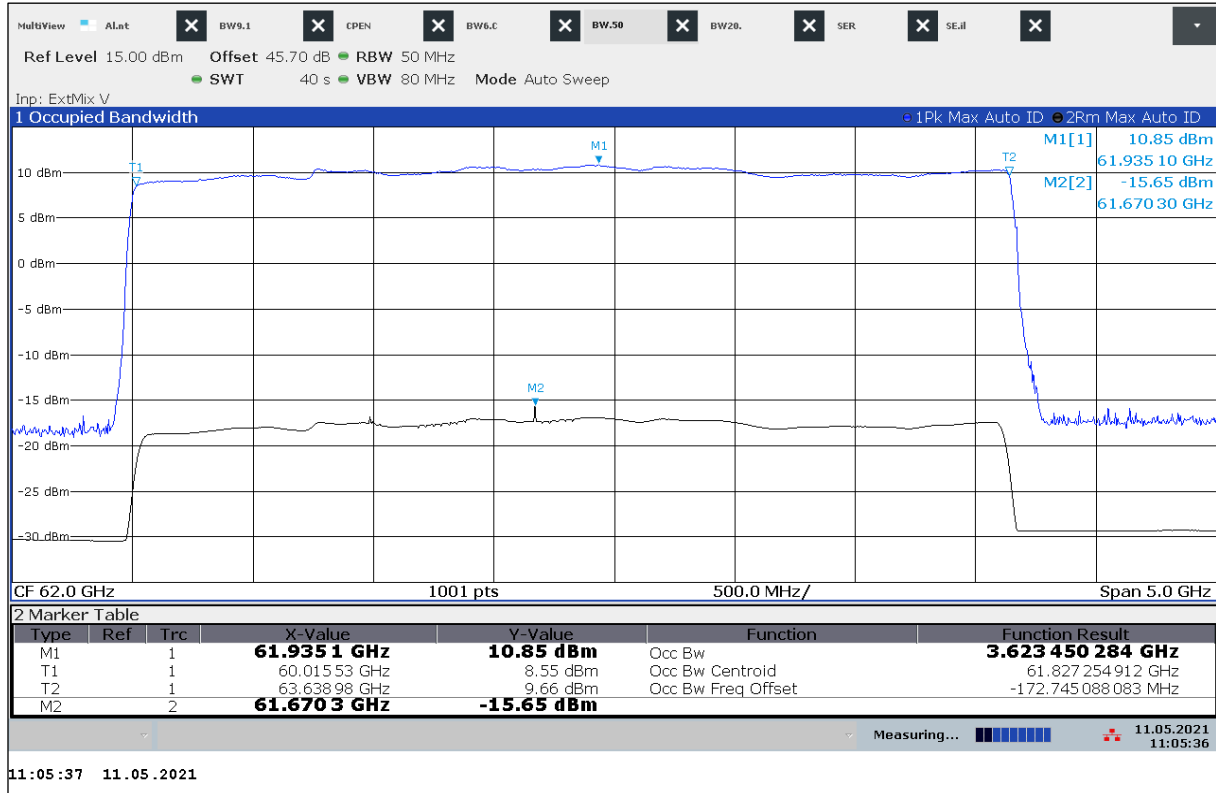
Plot 36: Frequency Stability, Single Target Mode (STM), -40 °C / V min-max
