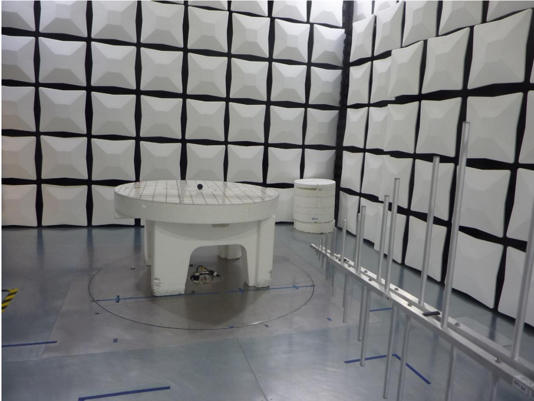
Figure 1: Test Setup for 30 MHz to 1 GHz (View 1)
