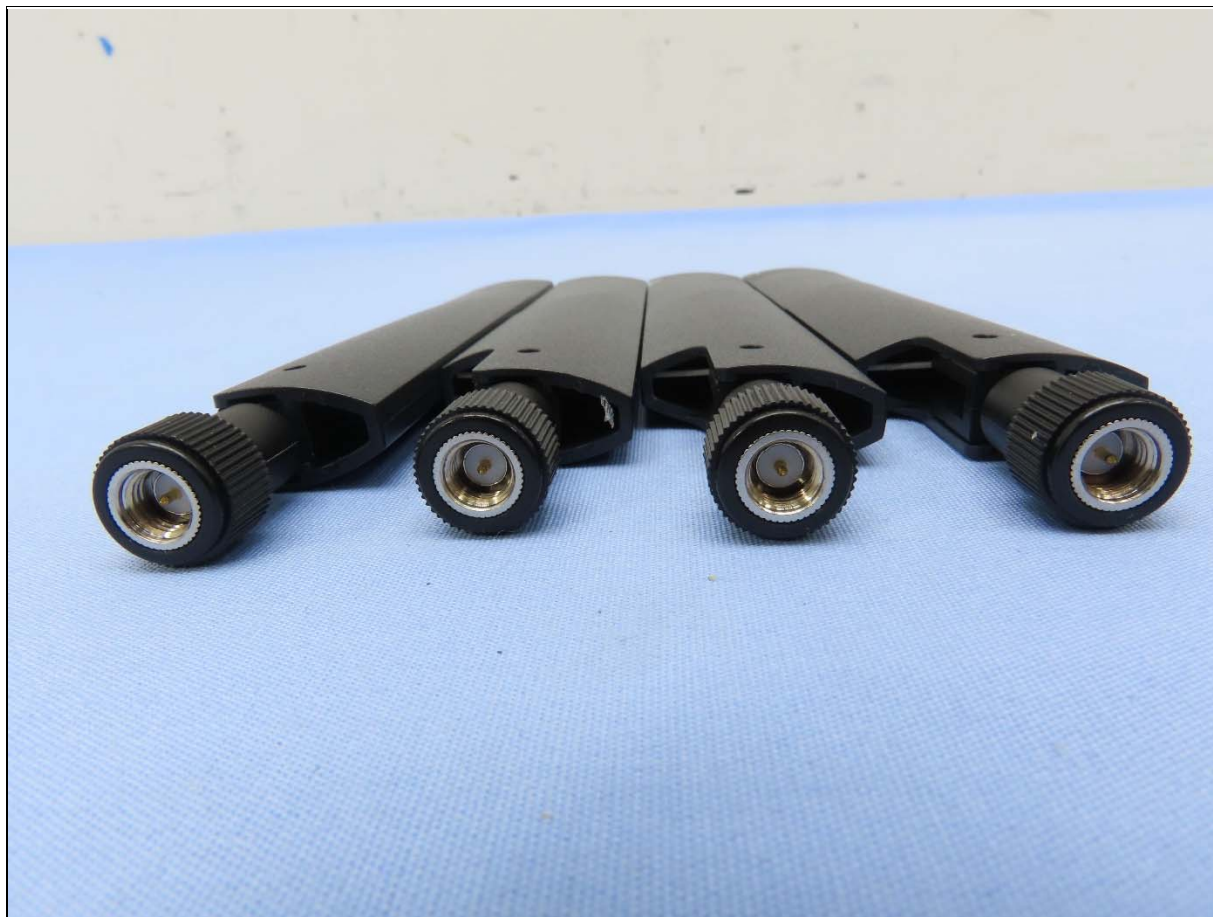
Cellular: Monopole Antenna (Brand: MaxTena, Model: NETZ 4IN1-5G)
