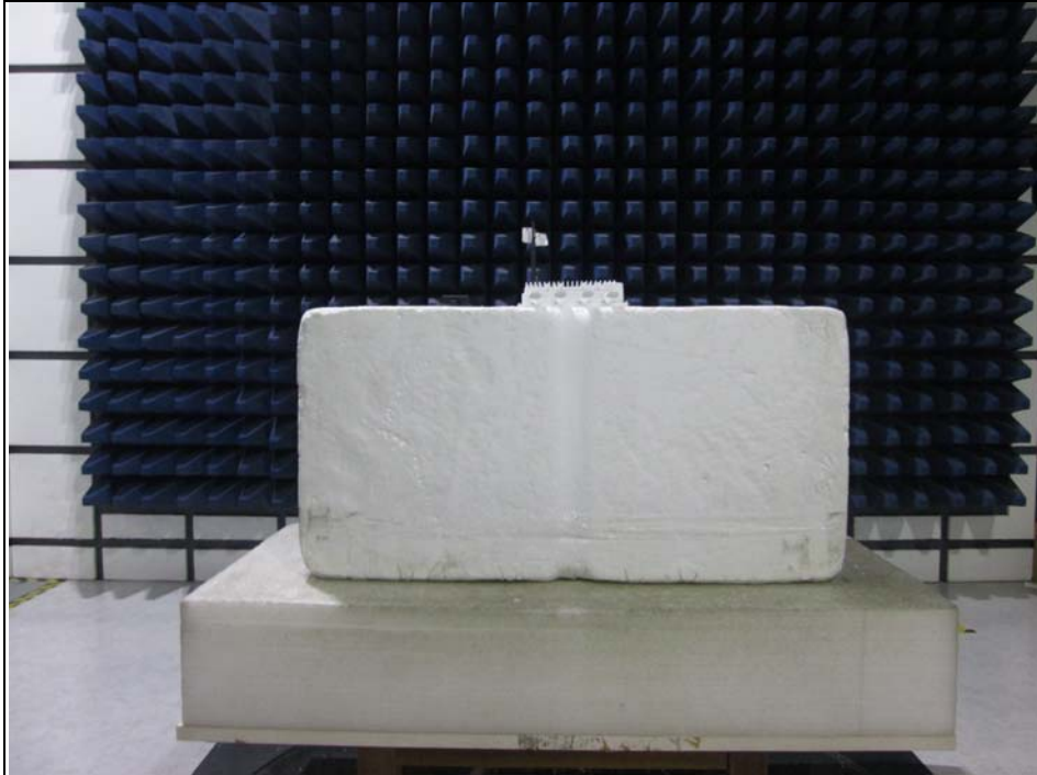
Radiated Emission Test (Above 1GHz) (X-plane)
