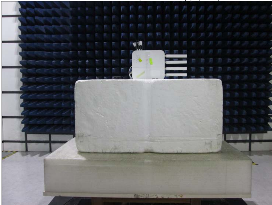
Radiated Emission Test (Above 1GHz) (Z-plane)
