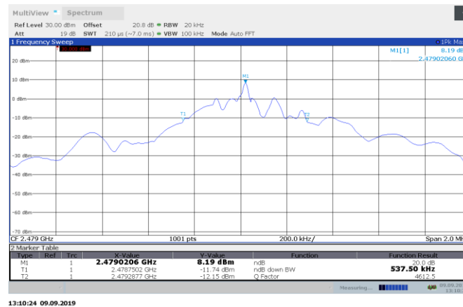
Figure 8.4-9: 20 dB bandwidth at 2479 MHz, Channel B
