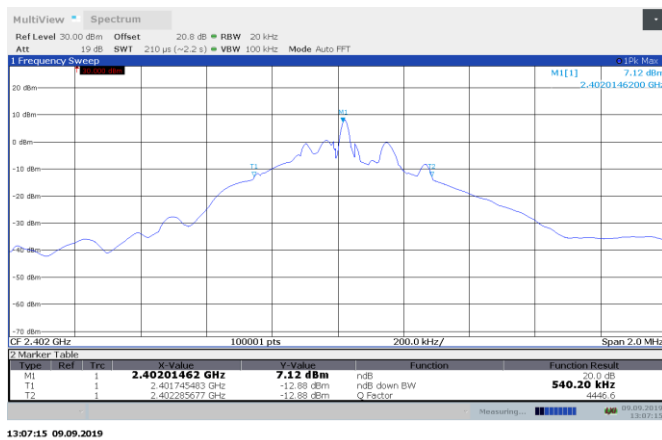
Figure 8.4-7: 20 dB bandwidth at 2402 MHz, Channel B
