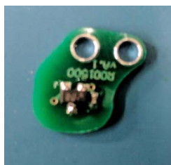
Figure 8: Hall Sensor Board, Front
