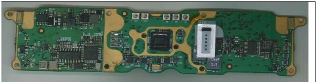
Figure 2: Main Board, Front
