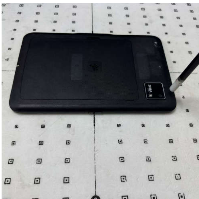
Bottom face-Top, Test Separation 2 mm
