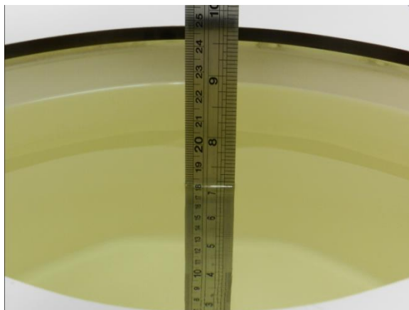
Fig 11.1 Photo of Liquid Height for Body SAR
