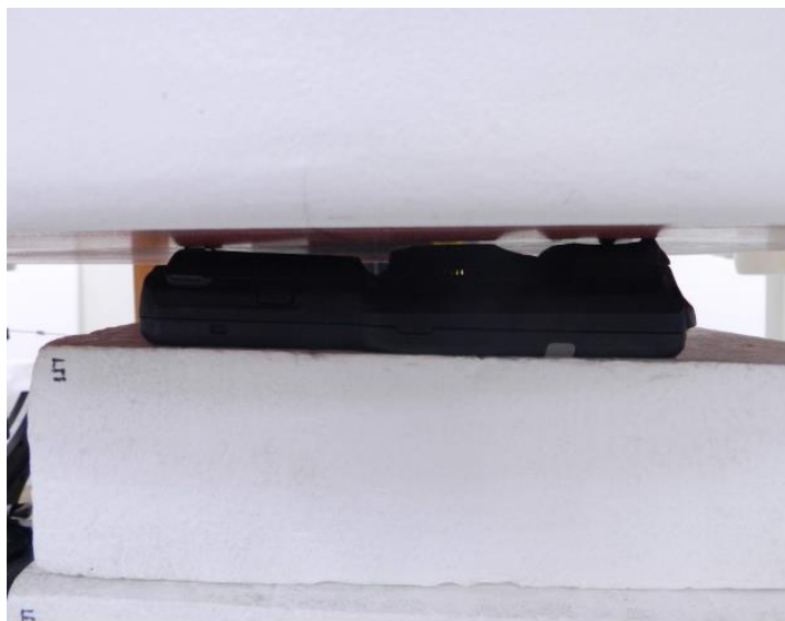
Extremity test mode for EUT Type 3 (cut off the pistol grip)
