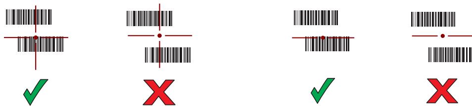
Figure 6 Pick List Mode with Multiple Barcodes in Aiming Pattern: Standard and Extended Range
