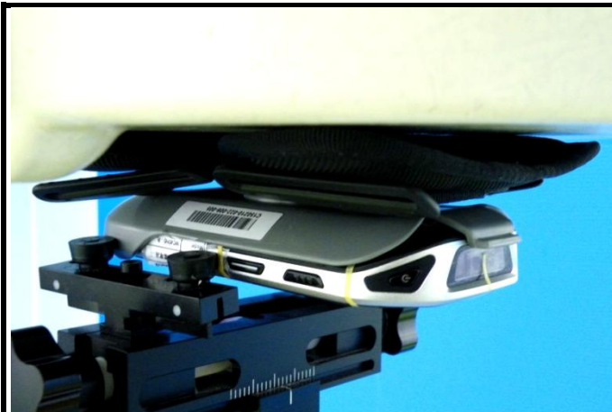
Rear Face of EUT with Holster 0 cm Gap
