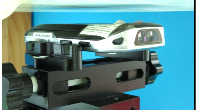
Rear Face of EUT with 1.5 cm Gap
