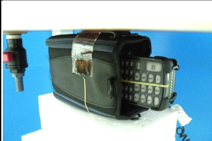
Right Side of EUT with 0 cm Gap (w/ Headset + Holster 2)
