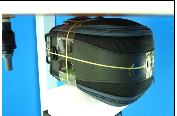
Left Side of EUT with 0 cm Gap (w/ Headset + Holster 2)
