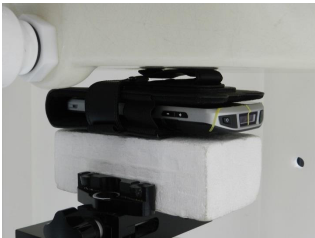
Front with Soft Holster, Test Separation 0 mm
