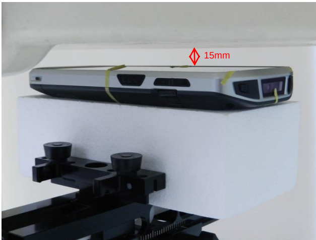
Front, Test Separation 15 mm
