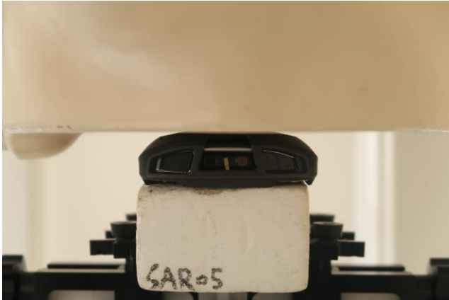
Back + Exoskeleton + Trigger Handle1, Test Separation 0mm
