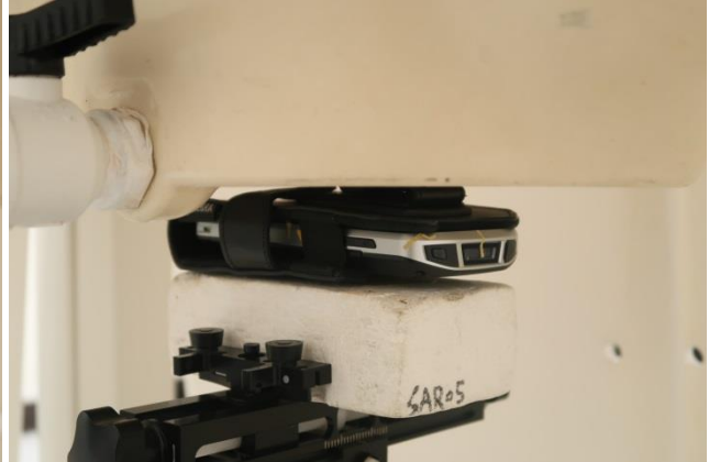
Front + Soft holster, Test Separation 0mm
