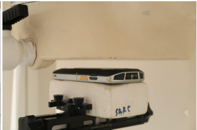
Back side, Test Separation 15mm
