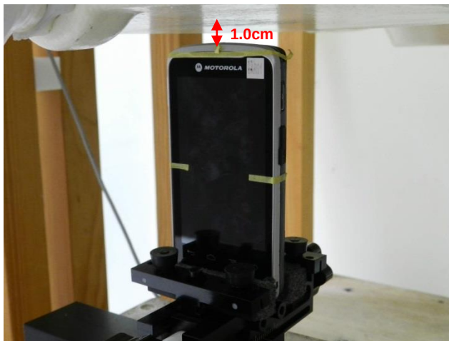
Top Side With Battery 1,Test Separation 1 cm
