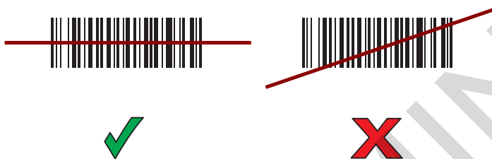
Figure 83: Linear Scanner Aiming Pattern
