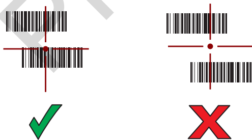
Figure 86: Pick List Mode with Multiple Bar Codes in Aiming Pattern
