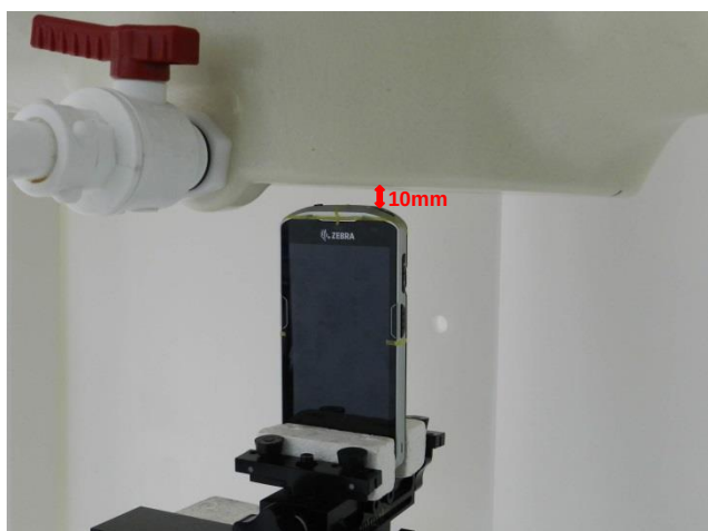
Top Side, Test Separation 10 mm
