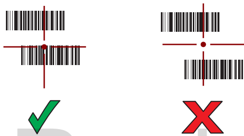
Figure 3-10 Pick List Mode with Multiple Bar Codes in Aiming Pattern
