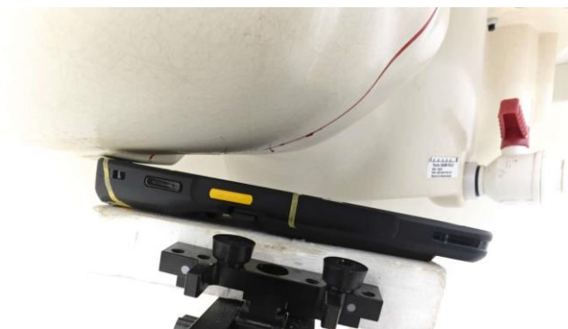
Right Tilted _ Extended, Test Separation 0 mm
