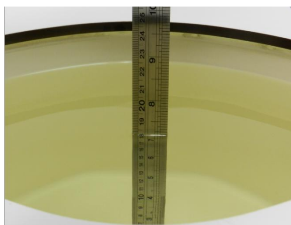
Fig 10.2 Photo of Liquid Height for Body SAR
