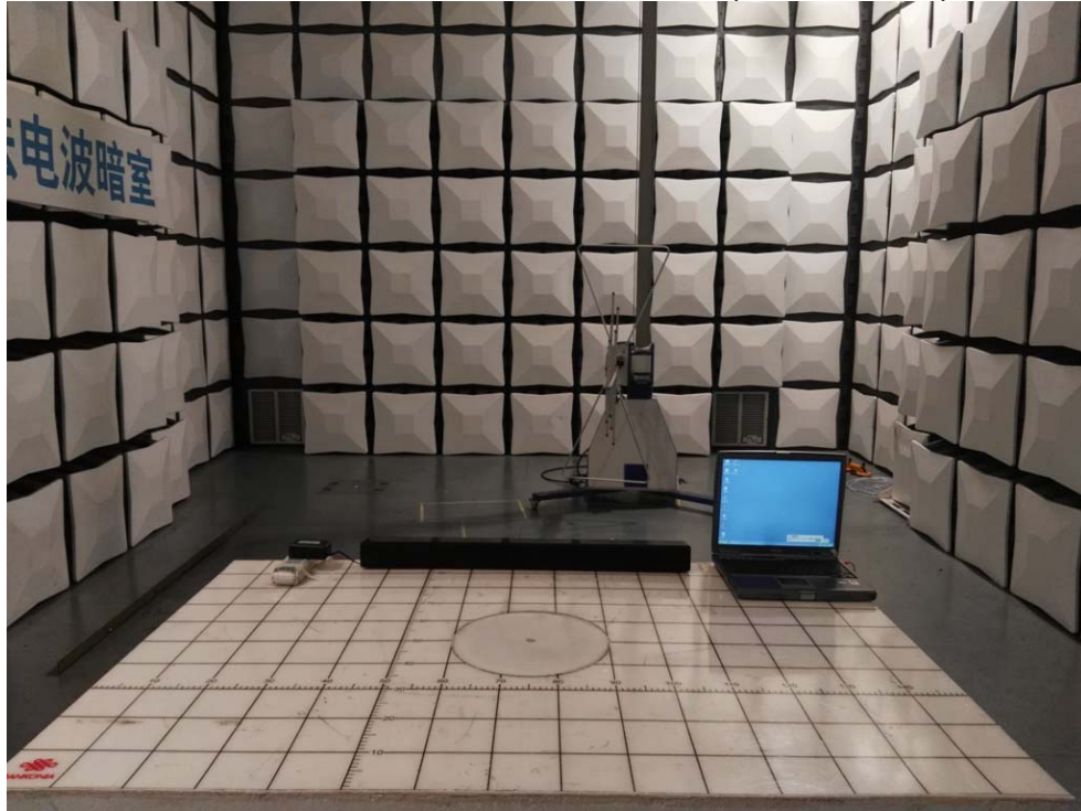
RADIATED RF MEASUREMENT SETUP (Above 1 GHz)
