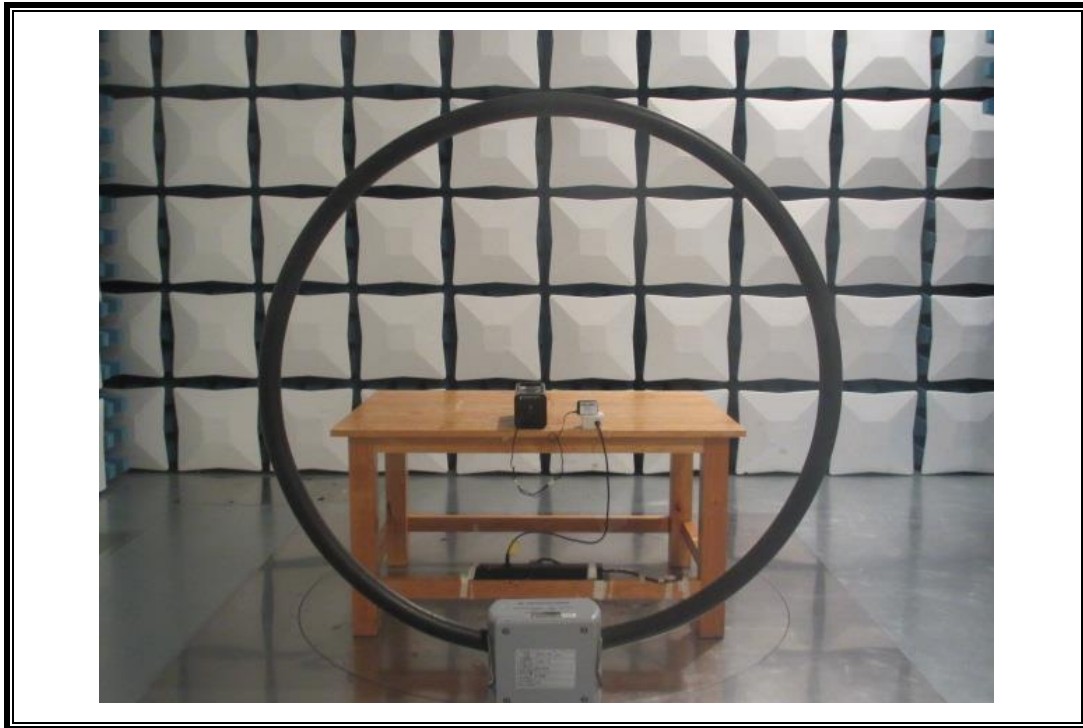
RADIATED RF MEASUREMENT SETUP (30MHz ~ 1 GHz)
