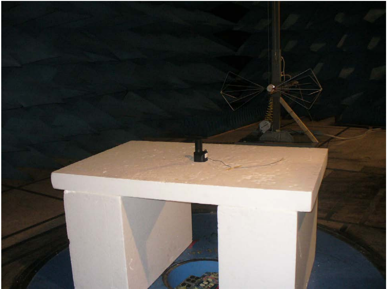
Figure 3: Radiated Emissions – Back View – 30 MHz – 200 MHz
