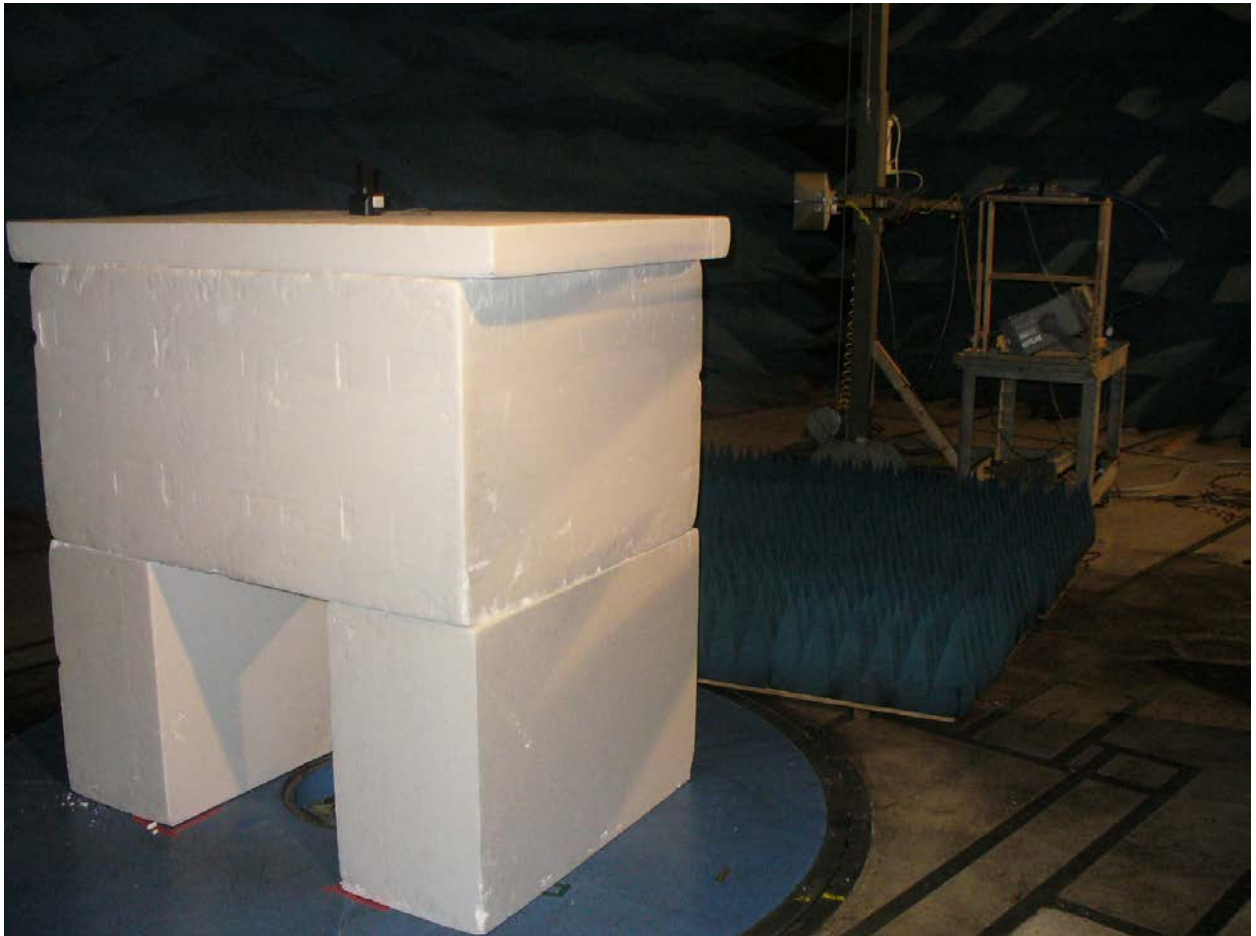
Figure 6: Radiated Emissions – Back View – Above 1 GHz
