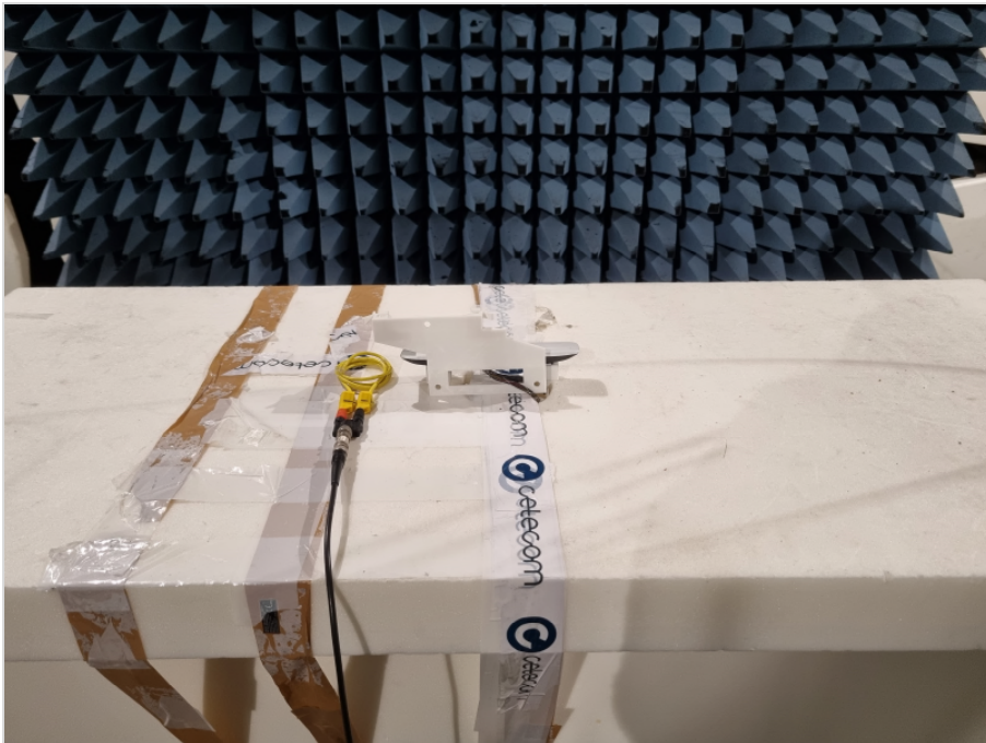
Photograph 3: EUT test setup in the semi anechoic chamber, close up view_EUT elevation 90°, EUT in TX mode
