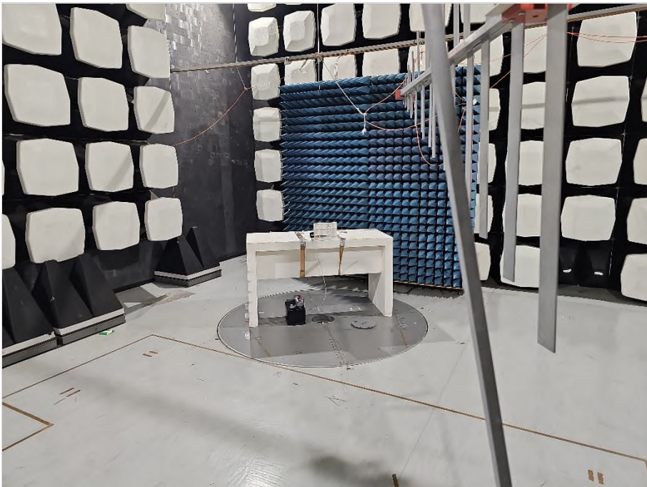
Photograph 8: EUT test setup in the anechoic chamber > 30 MHz, TXRX-mode, overview_EUT elevation 90°
