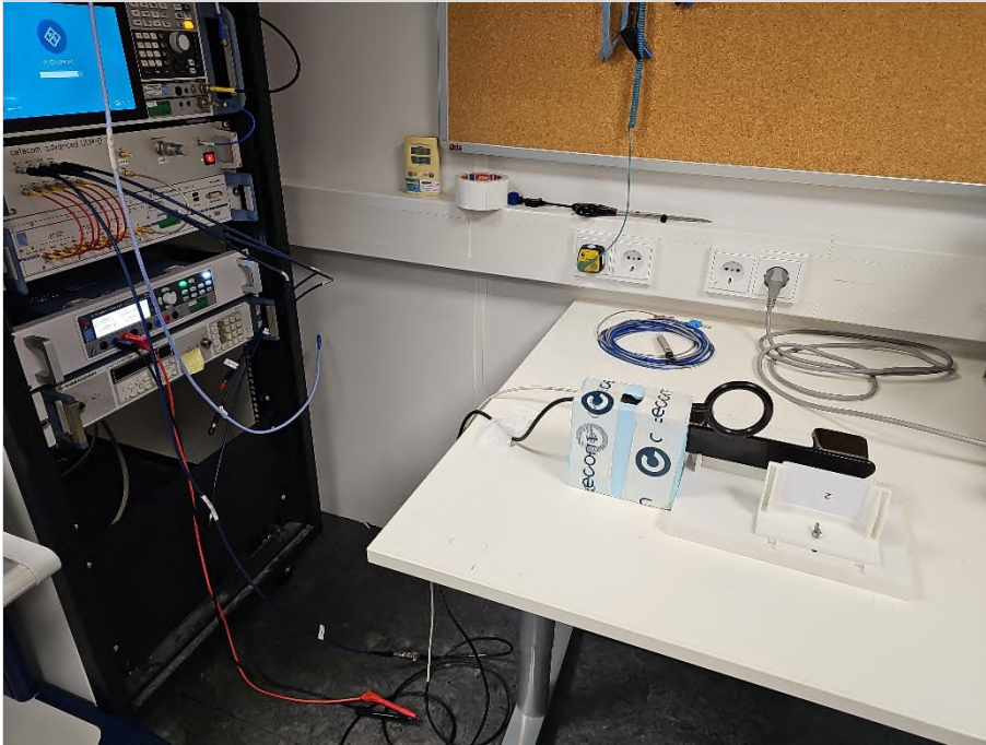
Photograph 1: EUT setup conducted measurement, overview
