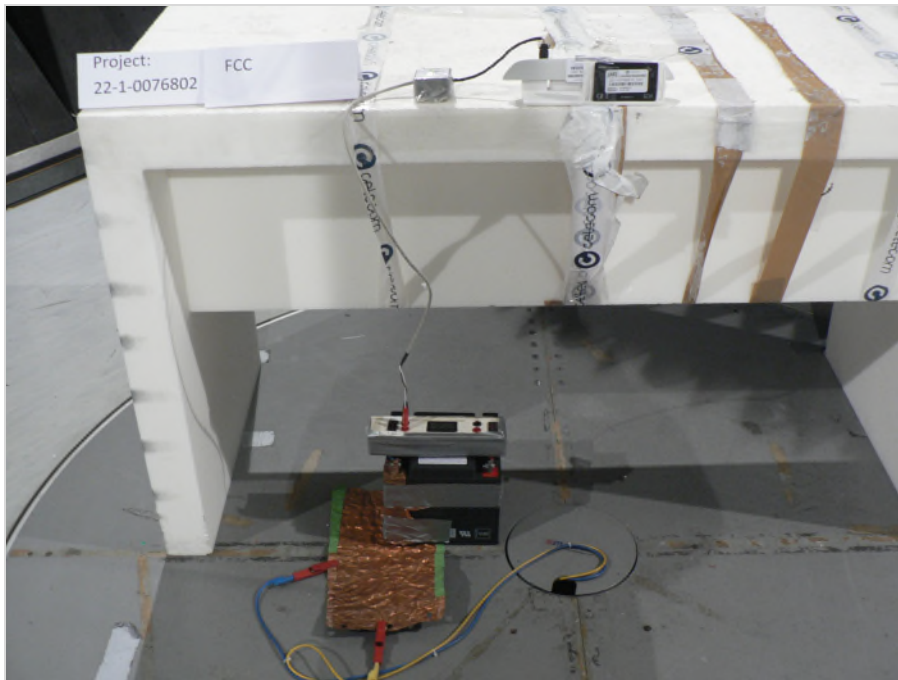
Photograph 7: Setup in the semi anechoic chamber, measurement >30 MHz, close up view, with NFC-Tag
