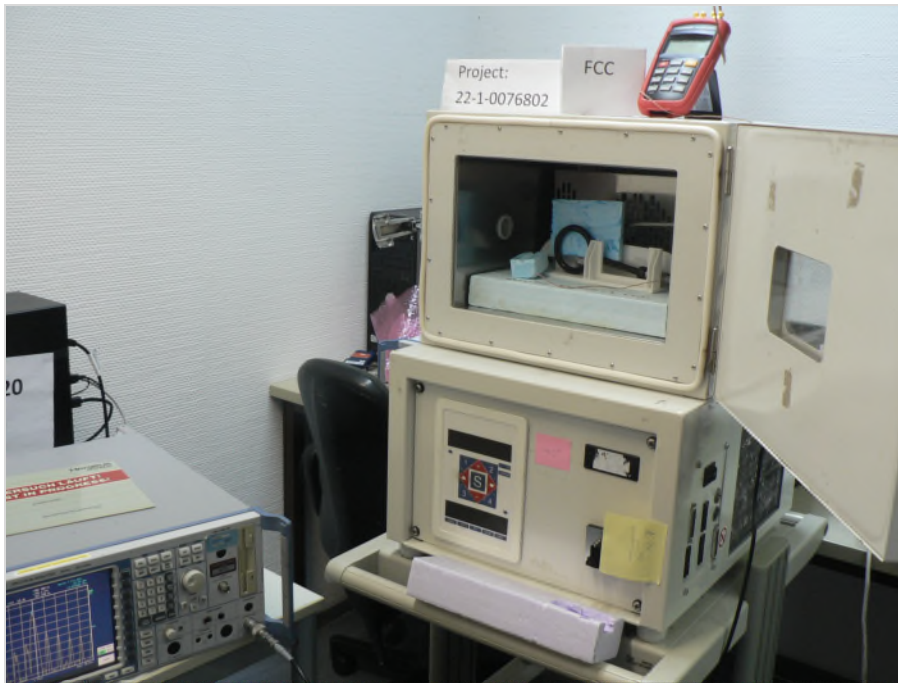
Photograph 3: Setup for extreme temperature measurement, overview
