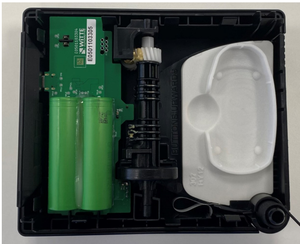
flinkey BLE enclosure lower part
