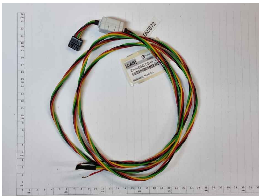
Photograph 2: CAB 1_CAN / Power cable
