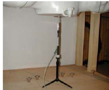
Figure 11.1 Dipole Verification Test Setup Diagram &amp; Photo
