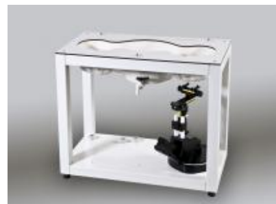
Figure 3.5 SAM Twin Phantom
